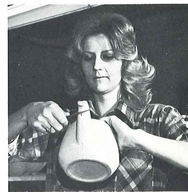
(4) Trimming with knife.
